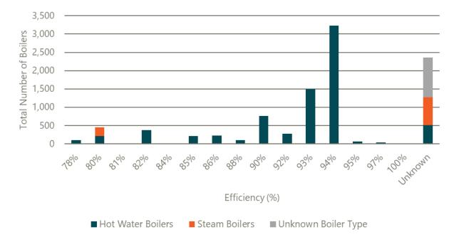
Figure 10: Number of Commercial Boilers by Rated Efficiency and Boiler Type (2019 CBSA)
