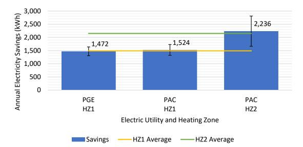
Chart 6: Electric savings for heat pump upgrades in site-built homes by electric utility & heating zone<sup>8</sup>
