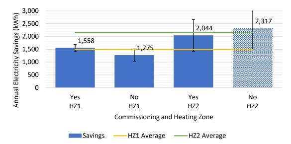
*Chart 8: Electric savings for heat pump upgrades in site-built homes by commissioning status and heating zone*<sup>9</sup>
