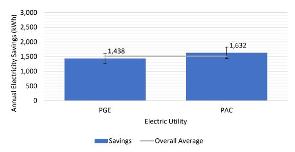
Chart 4: Electric savings for heat pump upgrades in site-built homes by electric utility
