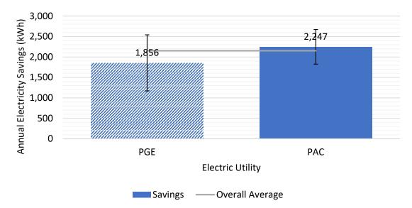
*Chart 5: Electric savings for heat pump upgrades in manufactured homes by electric utility<sup>7</sup>*
