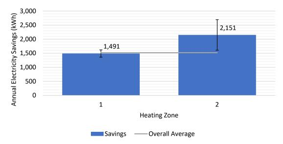
Chart 2: Electric savings for heat pump upgrades in site-built homes by heating zone
