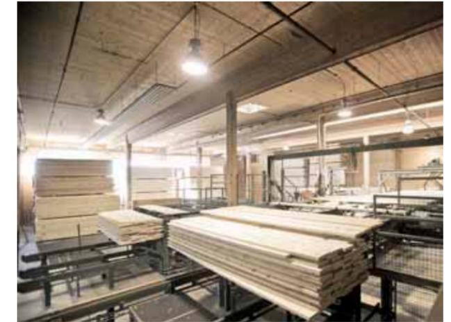
Cross-laminated timber is produced on a just-in-time basis
