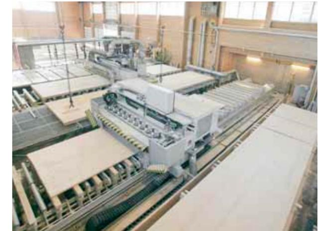
State-of-the-art CNC cutting machines facilitate both simple and highly complex patterns according to project requirements.
