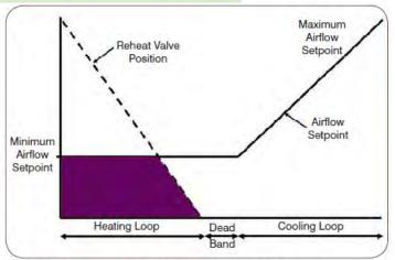
Figure 1: Conventional VAV reheat control diagram.
