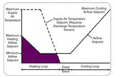
Figure 2: Dual maximum VAV reheat control diagram.
