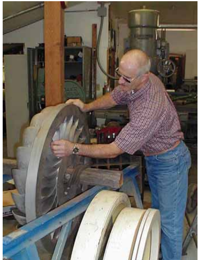
The author inspects a 990-pound, 22-inch pitch diameter Turgo-style runner for an 880 KW turbine.
