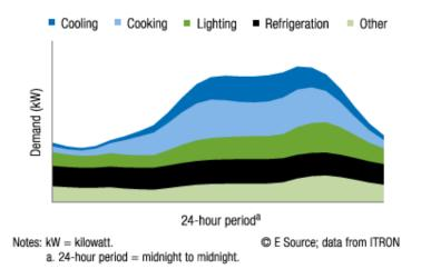
Figure 3. Example of load disaggregation for a commercial restaurant15
