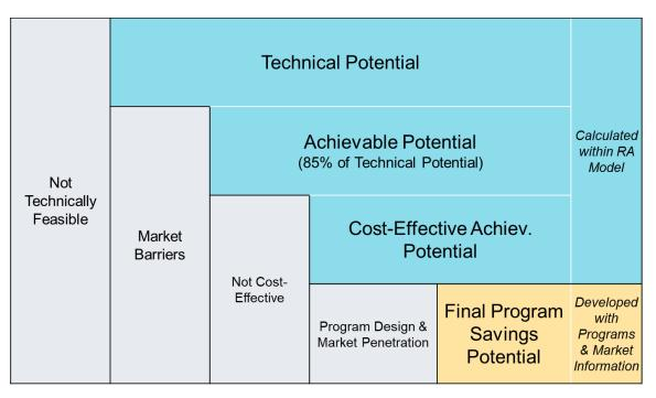
Figure 4: Types of Energy Savings Potential to Come out of Resource Assessment Modeling Process
