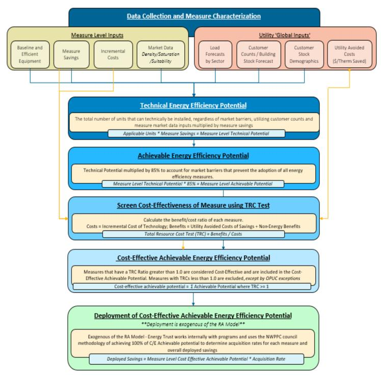
Figure 1: 20-year Energy Efficiency Forecast Development Process
