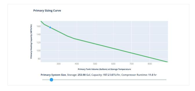
Figure 11: Ecosizer capacity curve with selection example
