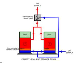
Figure 8: Multi-pass integrated HPWH system without hot water recirculation
