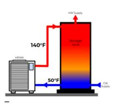
**Figure 1:** Single-pass: Heats water to the storage setpoint temperature in a single water pass through the refrigeration circuit, typically a 70°F to 100°F temperature lift in a single cycle
