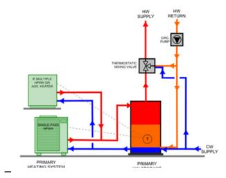
**Figure 6:** Single-pass primary HPWH system with hot water circulation returned to primary storage tank
