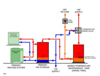
*Figure 3:* Single-pass primary HPWH system with series temperature maintenance tank (Swing Tank)
