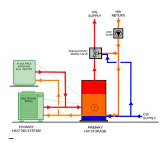
*Figure 5:* Multi-pass primary HPWH system with hot water return to primary storage
