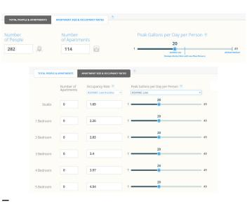
Figure 9: Ecosizer tool options for calculating daily hot water load
