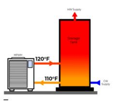
**Figure 2:** Multi-pass: Heats water to the storage setpoint temperature in a multiple water pass through the refrigeration circuit, typically a 10°F temperature lift for each cycle
