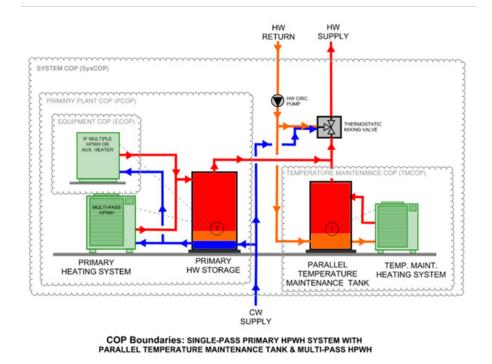
Figure 13: Elements of equipment and system efficiency ratings
