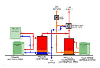
*Figure 4:* Single-pass primary HPWH system with parallel temperature maintenance tank and multi-pass HPWH (Parallel Loop Tank)
