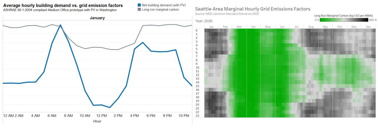
PV clearly changes the load shape in daylight hours...
